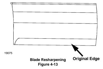
Check the blades for balance following grinding. A commercial balancing tool is available through most hardware supply stores, or balancing can be done by placing the blade on an inverted line punch or 1/2" bolt. Blade should not lean or tilt. Spin the blade slowly, blade should not wobble. If blade is out of balance, true it up before reinstalling.
